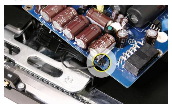
5. Disconnect the AC power inlet cable from the power supply. The cable is tucked neatly between the right pressure wall (black piece of molded plastic along the right side of the power supply) and the top of the logic board.
